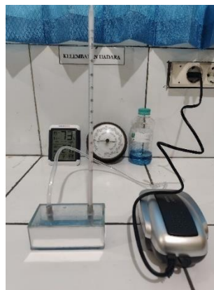
Gambar 6. Uji coba prototype dew point hygrometer
